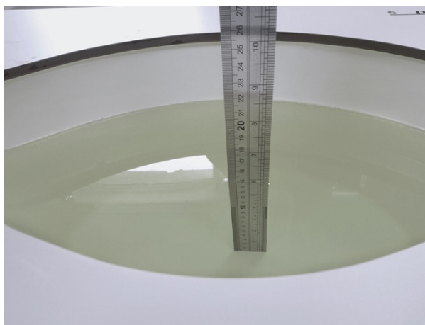
Liquid depth in the body phantom (2450MHz)
