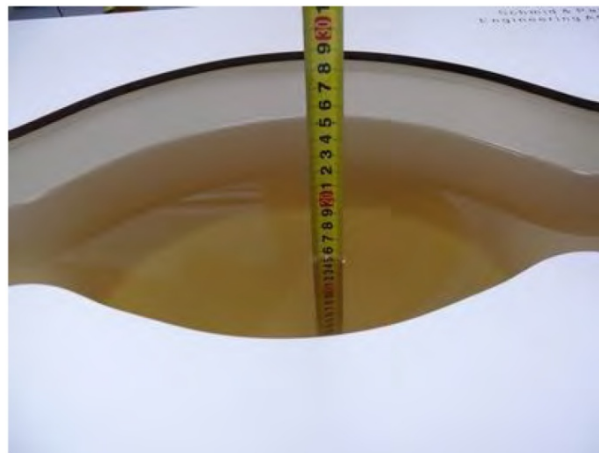
Liquid depth in the body phantom (835MHz)
