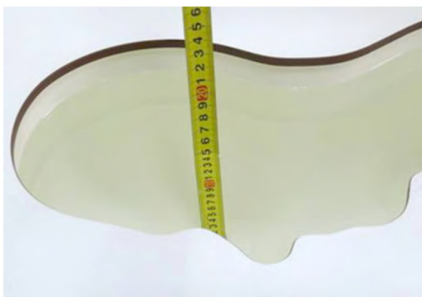
Liquid depth in the head phantom (835MHz)
