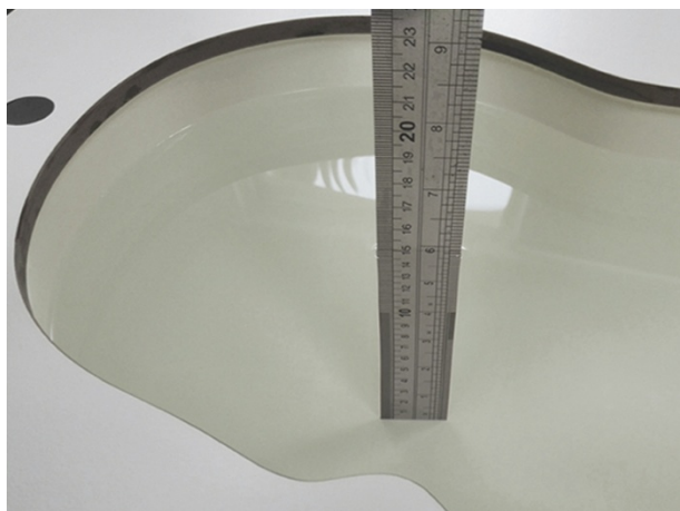
Liquid depth in the head phantom (2450MHz)
