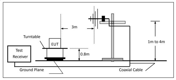
(c) For radiated emissions above 1000MHz
