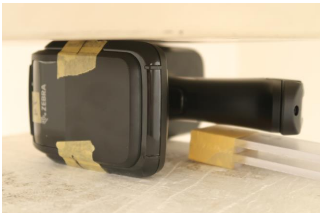
Right Side, Test Separation 0 mm
