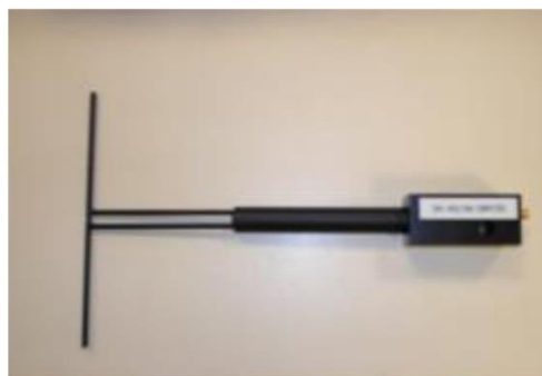
Figure 1 – Satimo COMOSAR Validation Dipole
