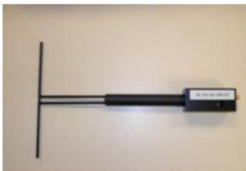
Figure 1 – Satimo COMOSAR Validation Dipole
