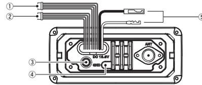
When connecting the external speaker, GPS, DC power supply, computer and navigation device by the rear panel cable end, cover the connectors and cables with rubber vulcanizing tape as below, to prevent water seeping into the transceiver.
