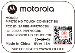
BU Label Size: 32x22.3mm Material: White label with matt lamination.
