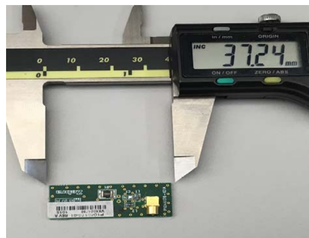
RFID Antenna Top View
