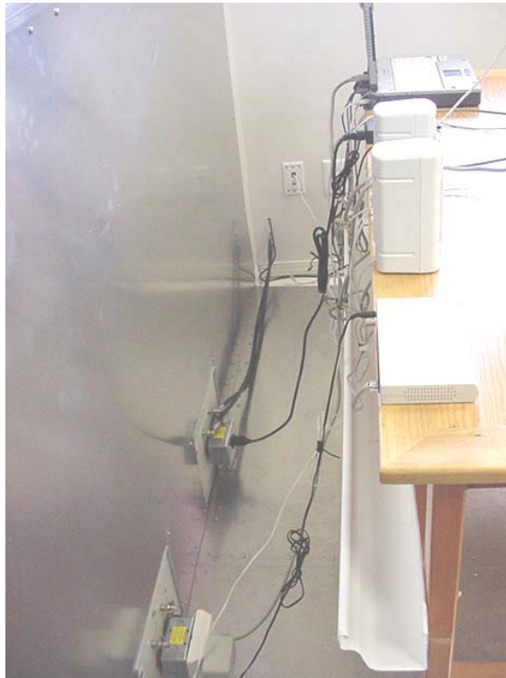
Photograph B-2 – AC Powerline Conducted Emission Cable Placement
