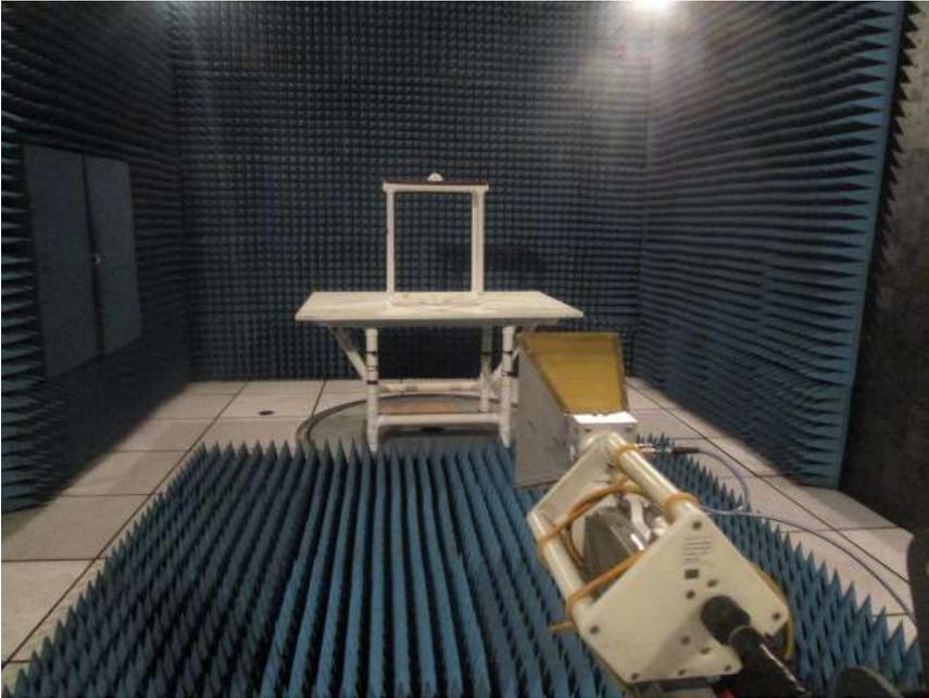
RADIATED EMISSIONS TEST SETUP 18 TO 25 GHZ
