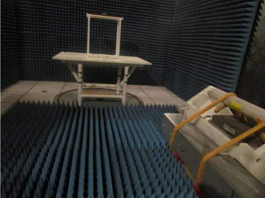
ANTENNA CONDUCTED TEST SETUP
