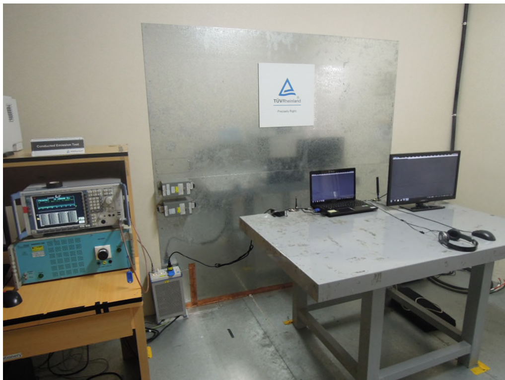
Photograph 22: Set-up for Mains Conducted testing (Front View)
