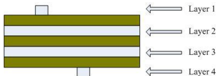
Figure 6-1-1-1 Application Board Layer Stack Up
