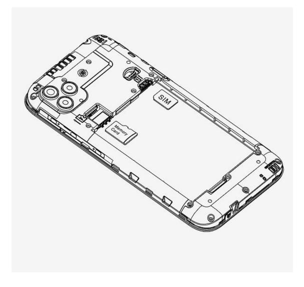
When inserting your card tray, make sure that the card is level and that the card is aligned correctly.
