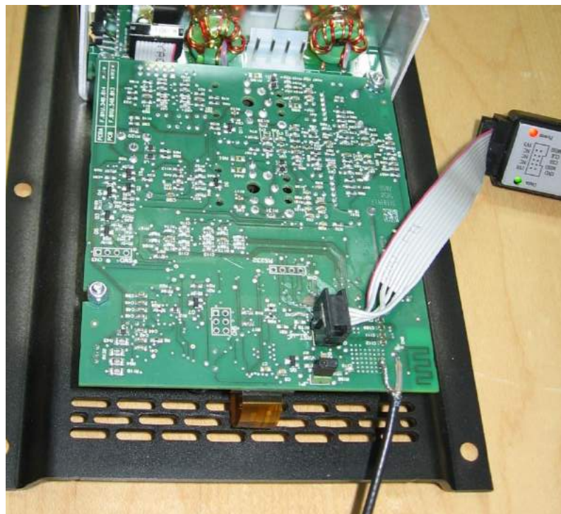
spurious emission conducted with spectrum analyzer
