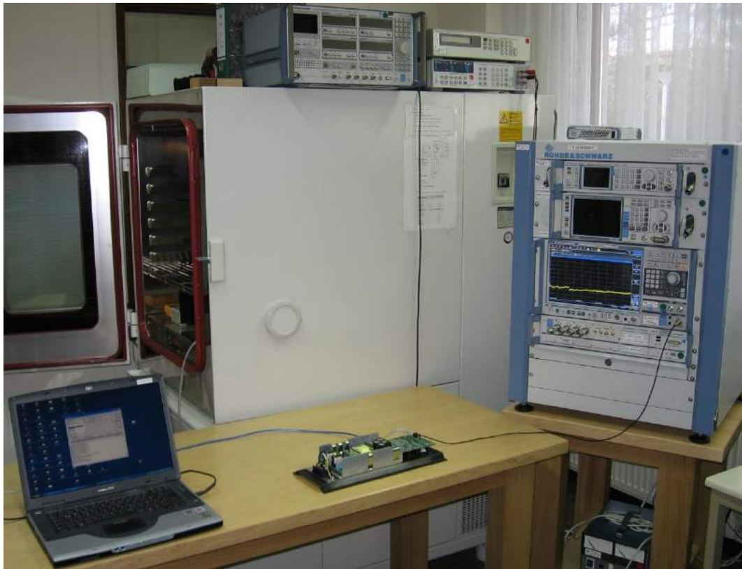
spurious emission conducted with spectrum analyzer
