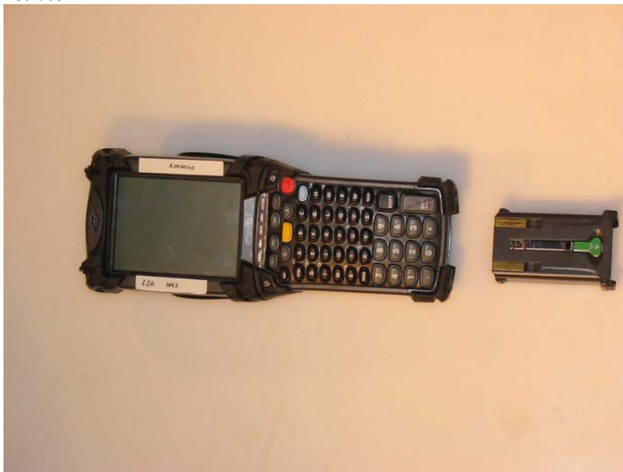
Figure 4 – MC9063 with Battery Removed
