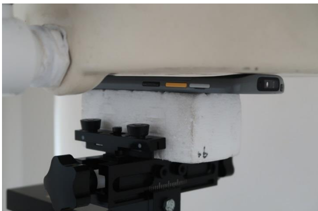
Back, Test Separation 0 mm
