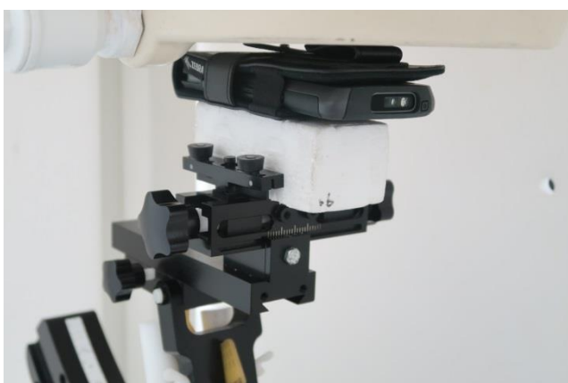
Back (Soft holster + Rigid Holster), Test Separation 0 mm
