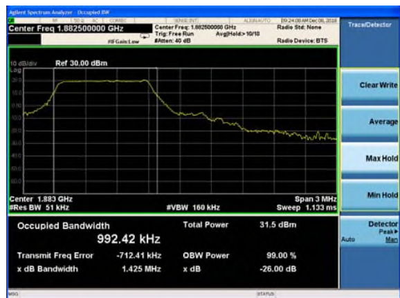
LTE Band 25 10MHz 16QAM CH-Middle
