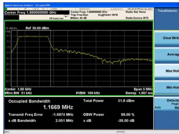
LTE Band 2 5MHz QPSK CH-Middle
