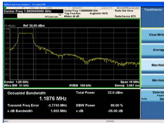
LTE Band 2 15MHz QPSK CH-Middle
