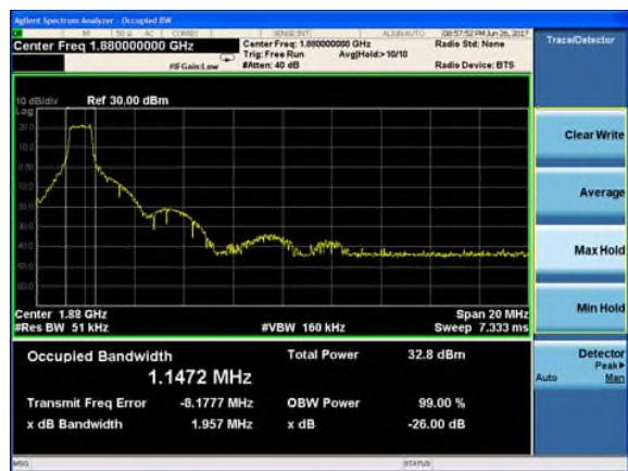
LTE Band 2 20MHz 16QAM CH-Middle
