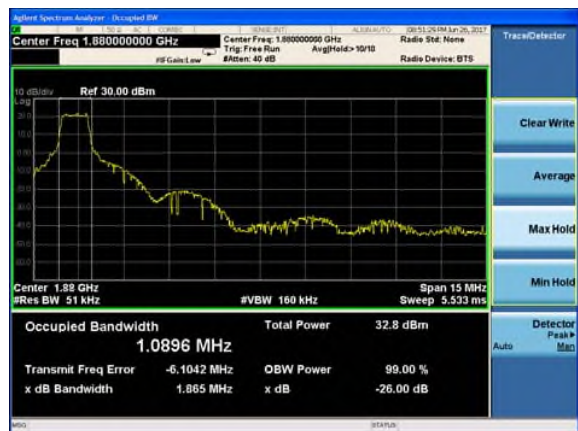
LTE Band 2 20MHz 16QAM CH-Middle
