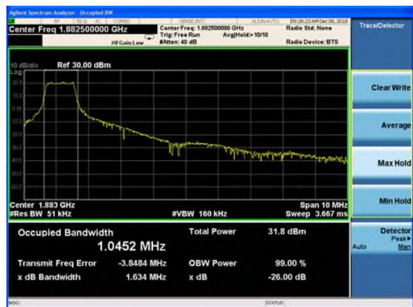
LTE Band 25 20MHz 16QAM CH-Middle
