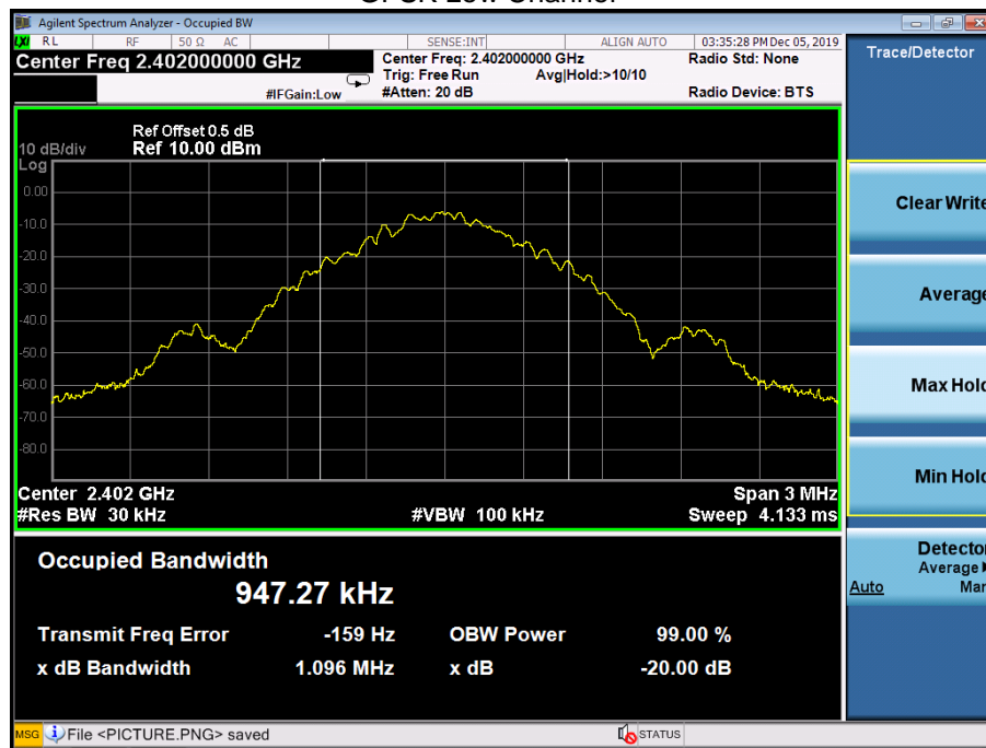
Test plots GFSK Low Channel
