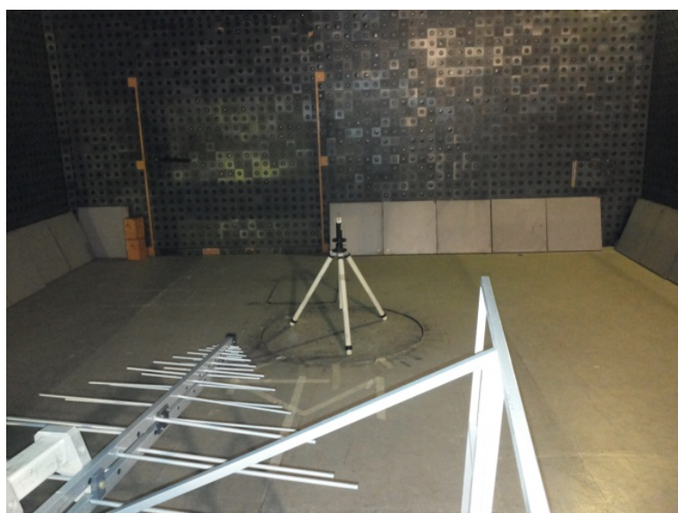
Photograph 8.1.1 Setup for radiated emission measurements
