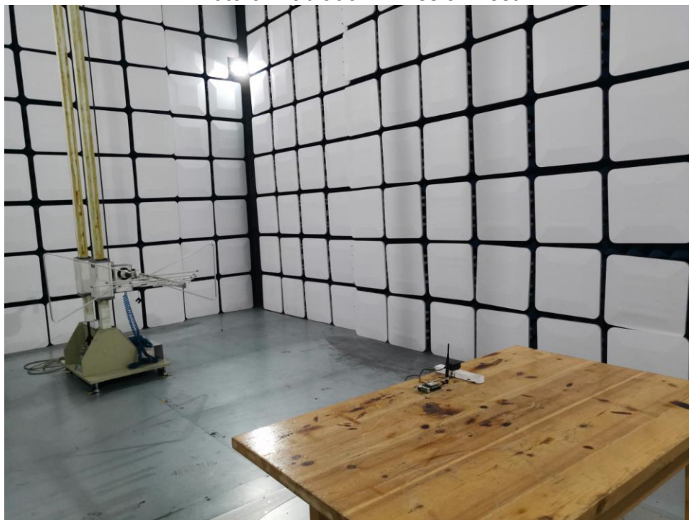
Photo of Radiation Emission Test
