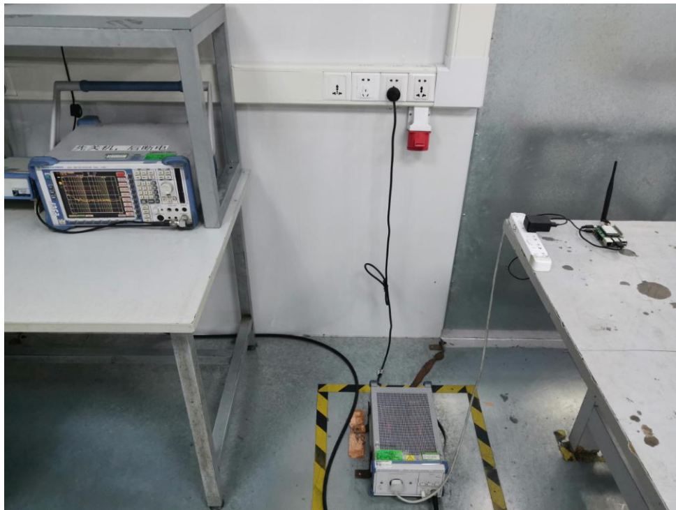
Photo of Conducted Emission Measurement
