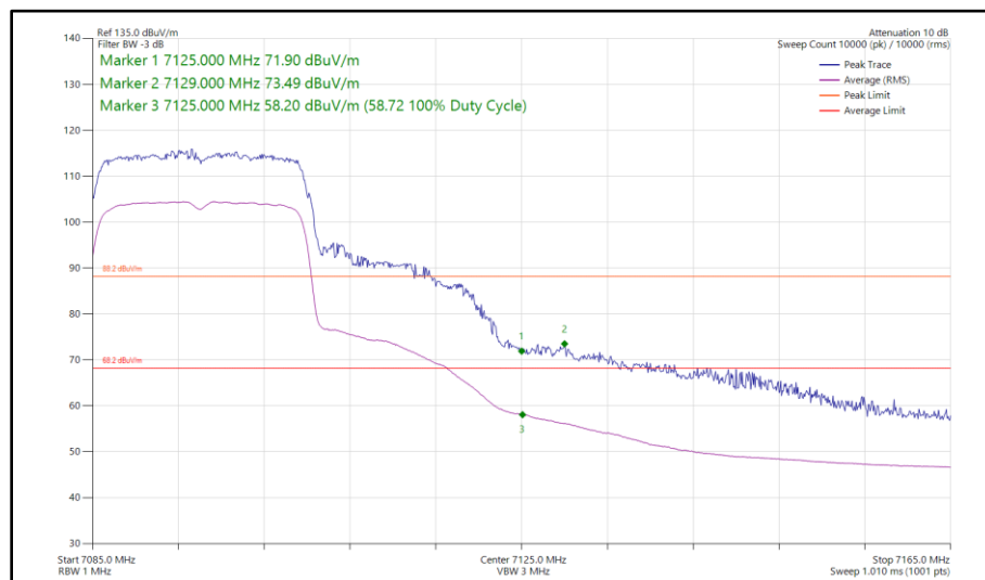
Figure 74 - 802.11ax HE20, SU, SISO, Core 1 - 7095 MHz Band Edge Frequency 7125 MHz
