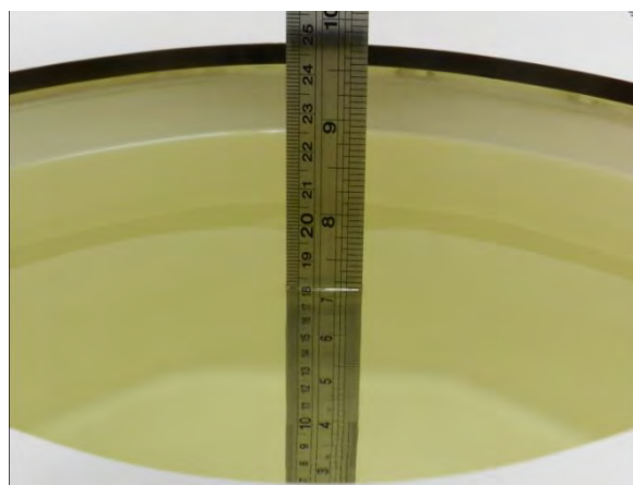
Fig 10.2 Photo of Liquid Height for Body SAR
