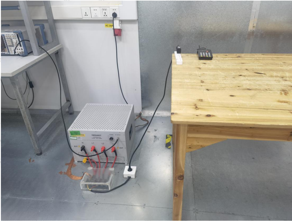
Photo of Conducted Emission Test
