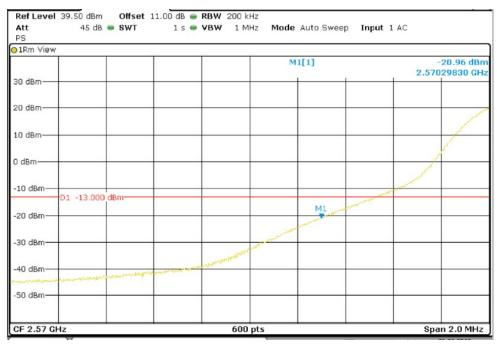
LTE QPSK MODULATION. RB = 1. Offset = Max. BW = 20 MHz
