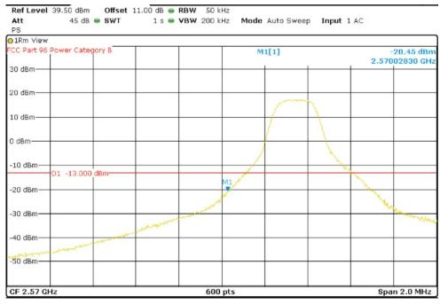
LTE QPSK MODULATION. RB = 1. Offset = Max. BW = 5 MHz
