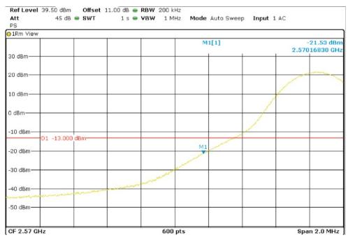
LTE QPSK MODULATION. RB = 1. Offset = Max. BW = 15 MHz
