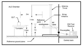
Radiated measurements > 1GHz
