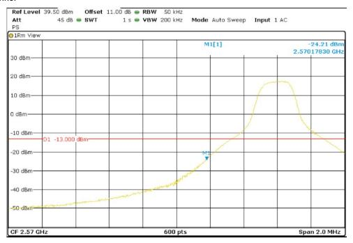
LTE QPSK MODULATION. RB = 1. Offset = Max. BW = 10 MHz
