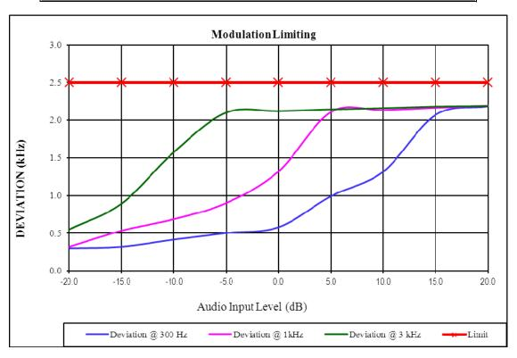
Note: the maximum frequency deviation is 2.2 kHz, which was declared by the manufactory.
