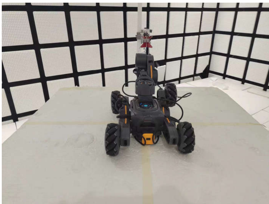
Radiated spurious emission Test Setup-2(Above 1GHz)
