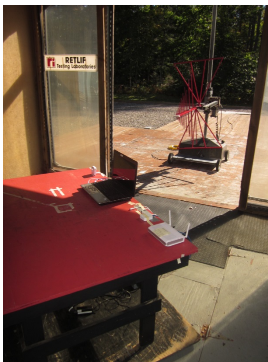
Vertical Antenna Polarization, 25 MHz – 1 GHz
