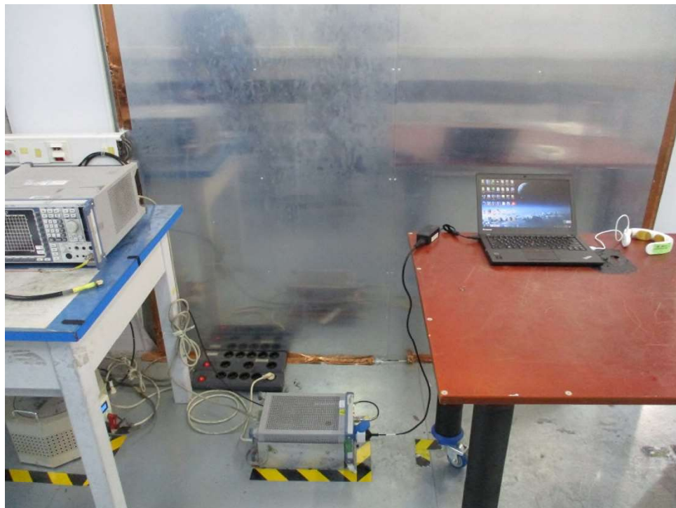
Photograph 4: Set-up for Conducted Emission on AC Mains
