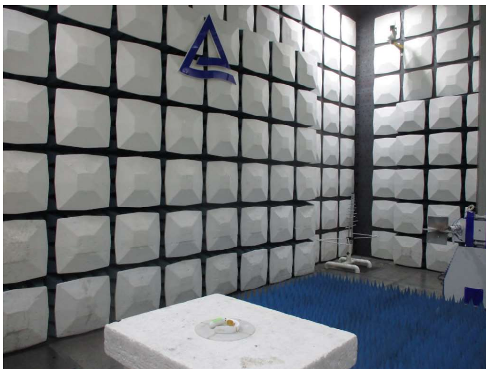
Photograph 2: Set-up for Radiated Spurious Emission, 1GHz - 18GHz
