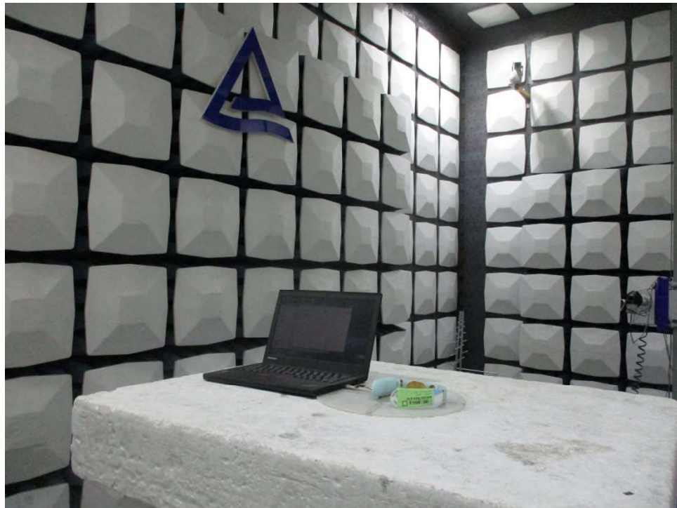
Photograph 4: Set-up for Conducted Emission on AC Mains
