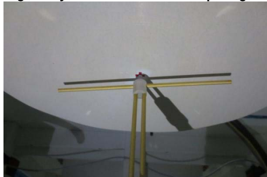
Fig.6.2 Photo of Dipole setup
