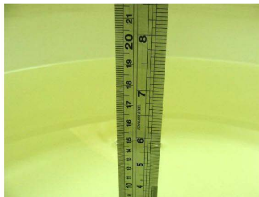
Fig 5.12 Photo of Liquid Height for Body SAR
