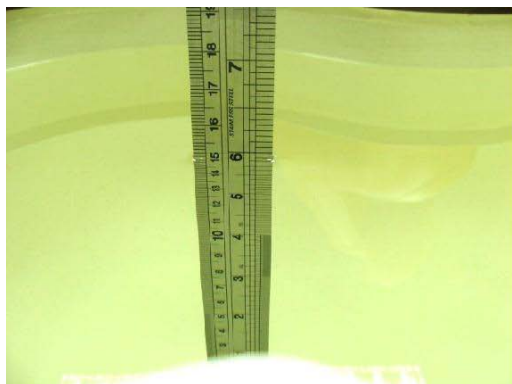
Fig 5.11 Photo of Liquid Height for Head SAR
