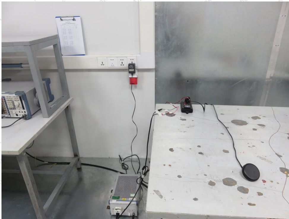
Photo of Power Line Conducted Emission Test
