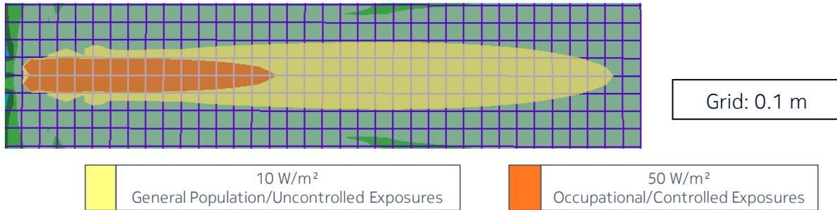
Figure 2 – Top view of the power density for the time-averaged maximum transmitted power of 2.8 W and the beam oriented in azimuth = 0° & elevation = 0° (EU/ICNIRP, Canada, Australia/NZ and US/related)
