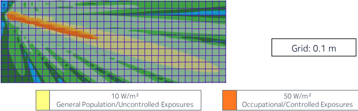
Figure 8 – Side view of the power density for the time-averaged maximum transmitted power of 2.8 W and the beam oriented in azimuth = 0° & elevation = +15° (EU/ICNIRP, Canada, Australia/NZ and US/related)
