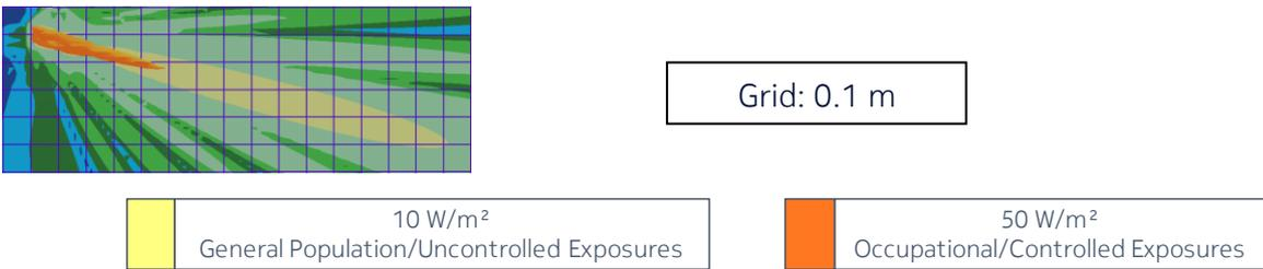
Figure 9 - Side view of the power density for the time-averaged actual maximum transmitted power of 0.7 W and the beam oriented in azimuth = 0° & elevation = +15° (EU/ICNIRP, Canada, Australia/NZ and US/related)
