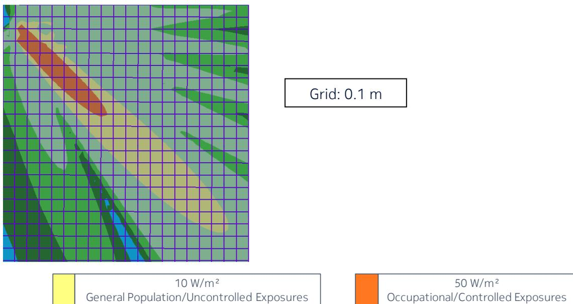
Figure 4 - Top view of the power density for the time-averaged maximum transmitted power of 2.8 W and the beam oriented in azimuth = -45° & elevation = 0° (EU/ICNIRP, Canada, Australia/NZ and US/related)
