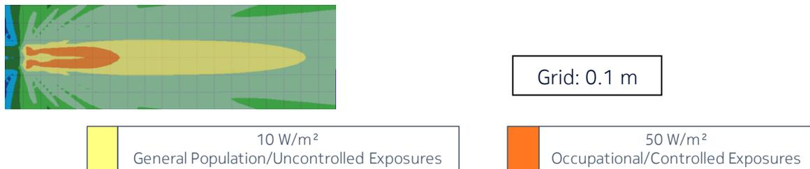
Figure 3 - Top view of the power density for the time-averaged actual maximum transmitted power of 0.7 W and the beam oriented in azimuth = 0° & elevation = 0° (EU/ICNIRP, Canada, Australia/NZ and US/related)
