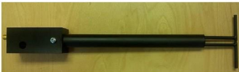
Figure 1 – MVG COMOSAR Validation Dipole
