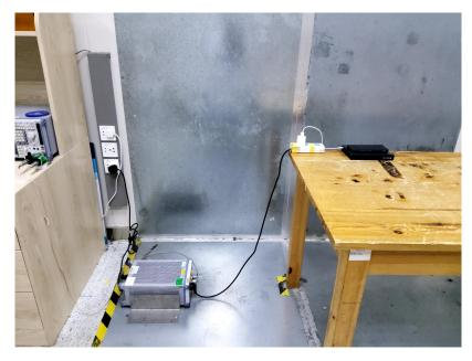
Radiated Emissions Test Frequency From 9KHz-30MHz
