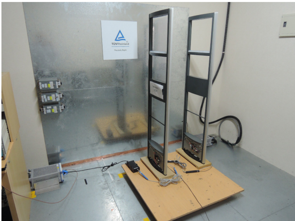
Photograph 5: Set-up for for Mains Conducted testing Front
