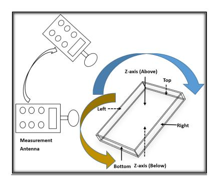
Note: The measurement antenna are moving and surrounding the EUT when performed the test, the test results recorded the highest values for each sides of the EUT (left/right/top/bottom/z-axis (Above)/z-axis (Below))
