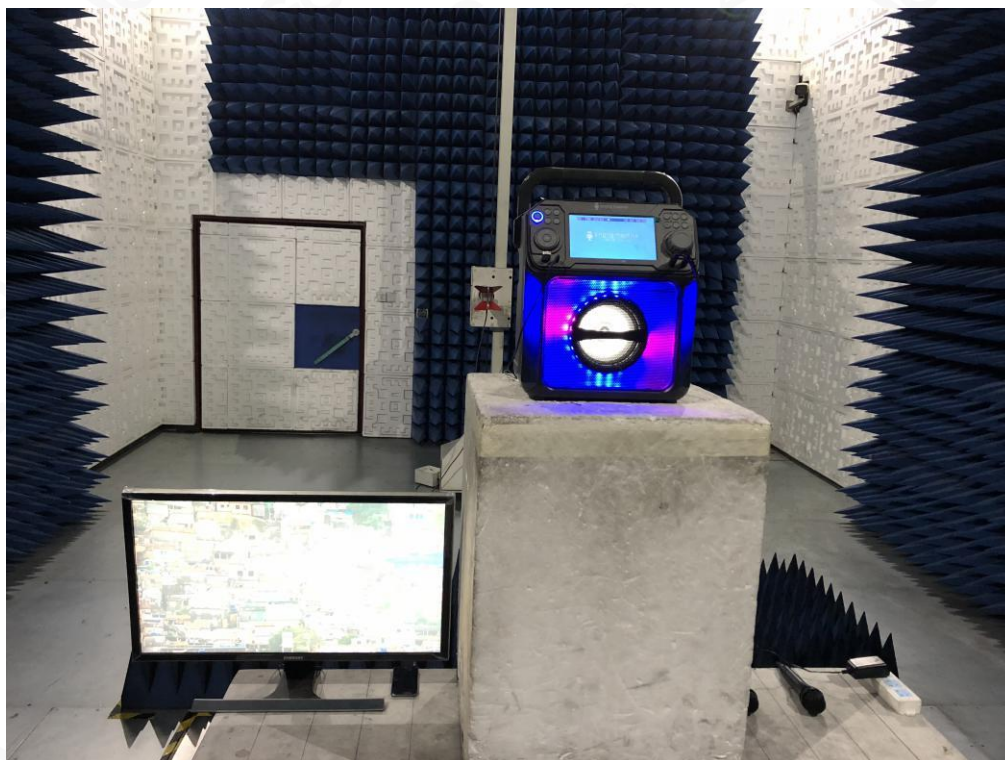
RADIATED EMISSION TEST SETUP ABOVE 1GHZ
