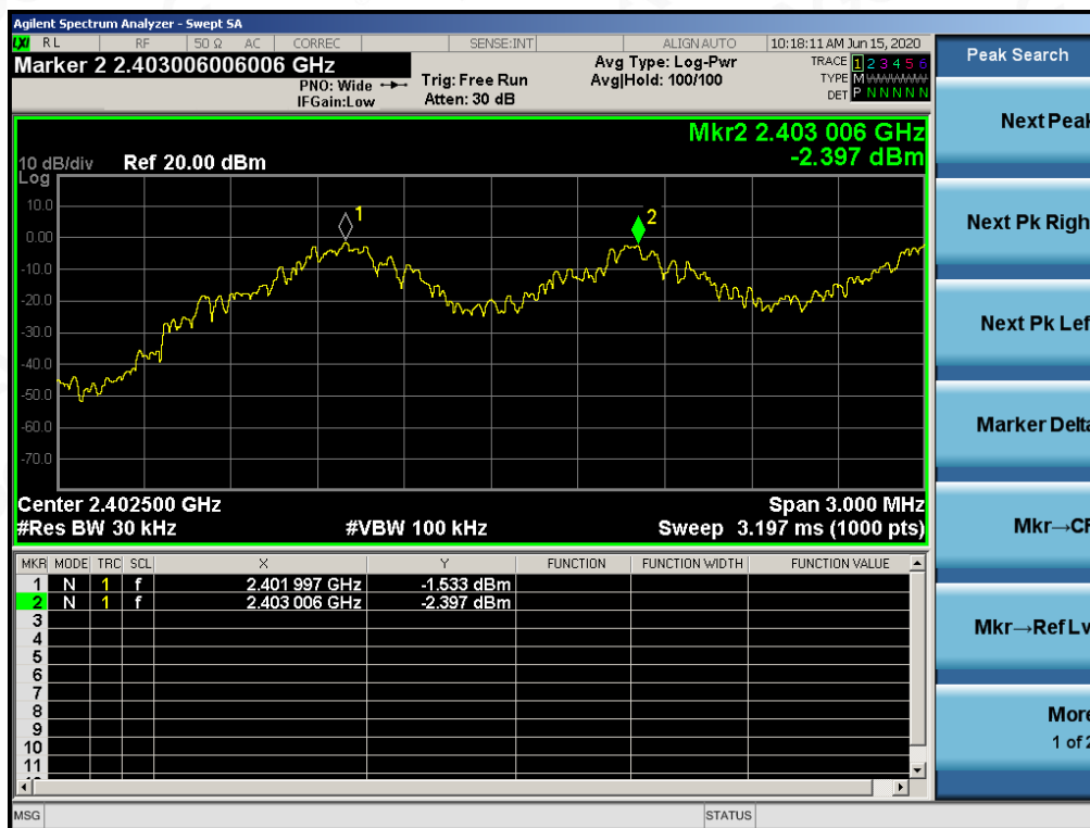
TEST PLOT FOR FREQUENCY SEPARATION
