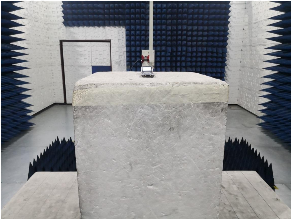
RADIATED EMISSION TEST SETUP ABOVE 1GHZ
