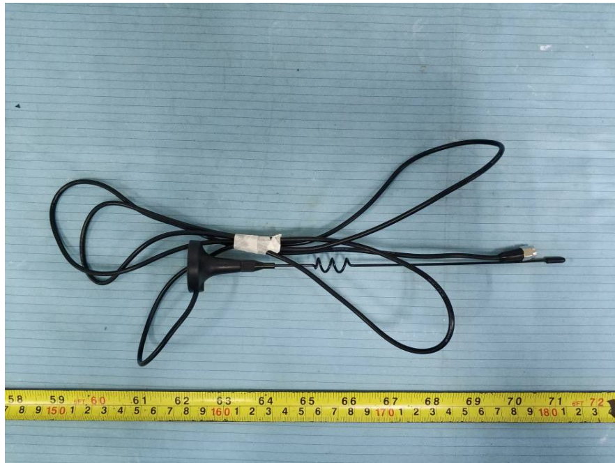
EUT – Wi-Fi Antenna View
