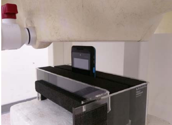
Fig.9 EUT Top side to flat phantom
