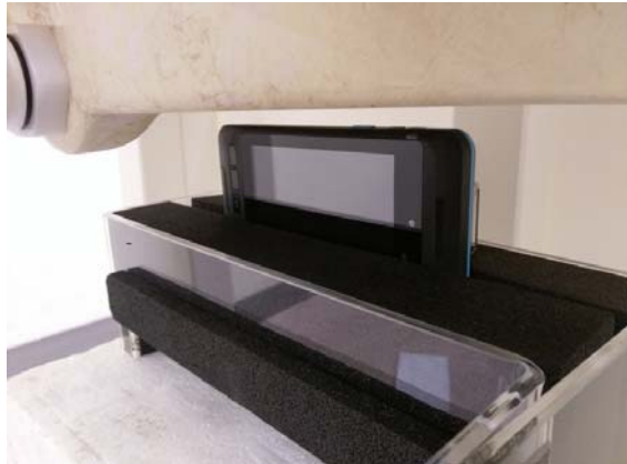
Fig.10 EUT Left side to flat phantom
