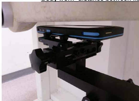
Fig.7 EUT Front side to flat phantom
