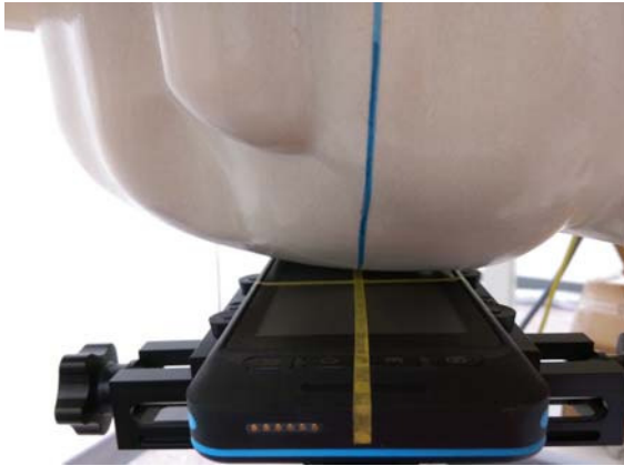
Fig.3 Right Head Section / Cheek-Touch Position
