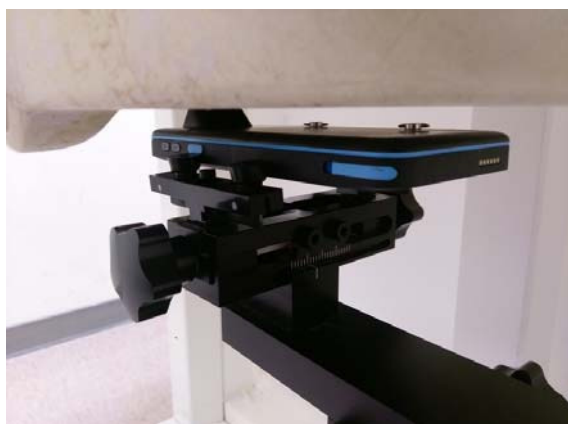
Fig.8 EUT Back side to flat phantom
