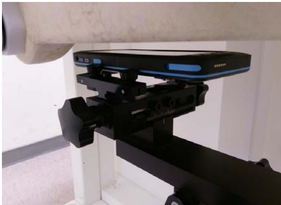
Fig.12 EUT Front side to flat phantom
