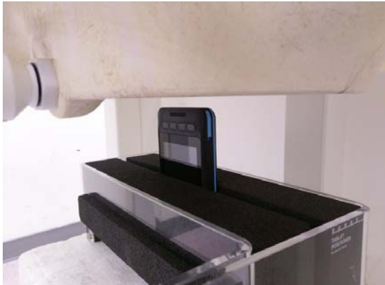
Fig.13 EUT Bottom side to flat phantom
