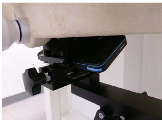
Fig.16 EUT Back side_WLAN to flat phantom
