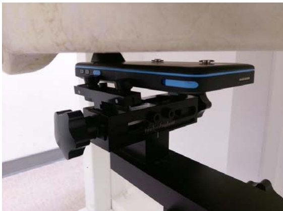
Fig.14 EUT Back side to flat phantom
