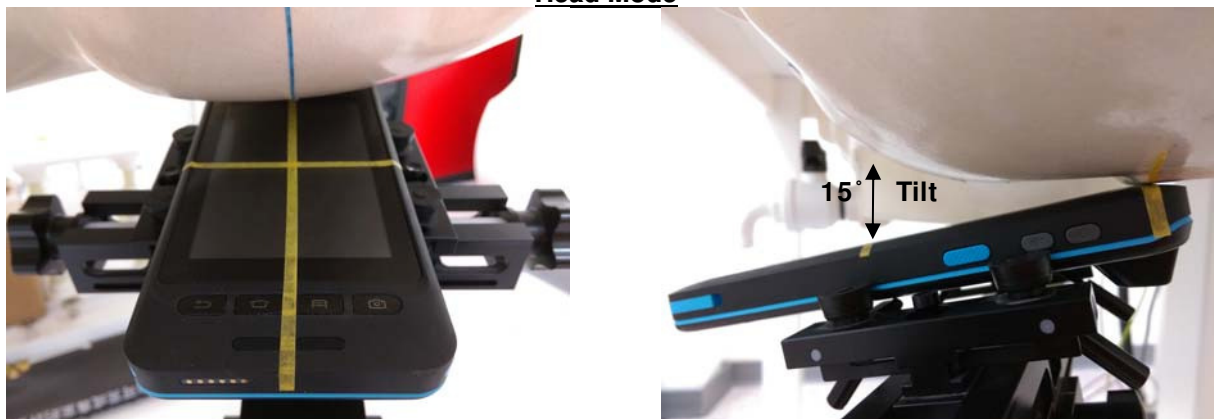
Fig.6 Left Head Section / Ear-Tilt Position(15°)
