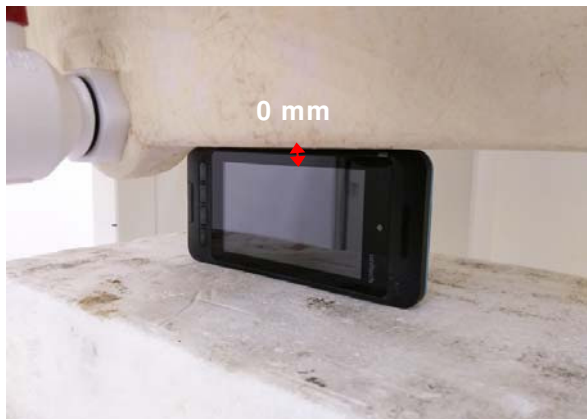
Fig.18 EUT Left side to flat phantom
