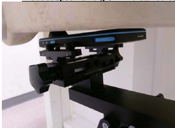
Fig.15 EUT Back side_WWAN to flat phantom
