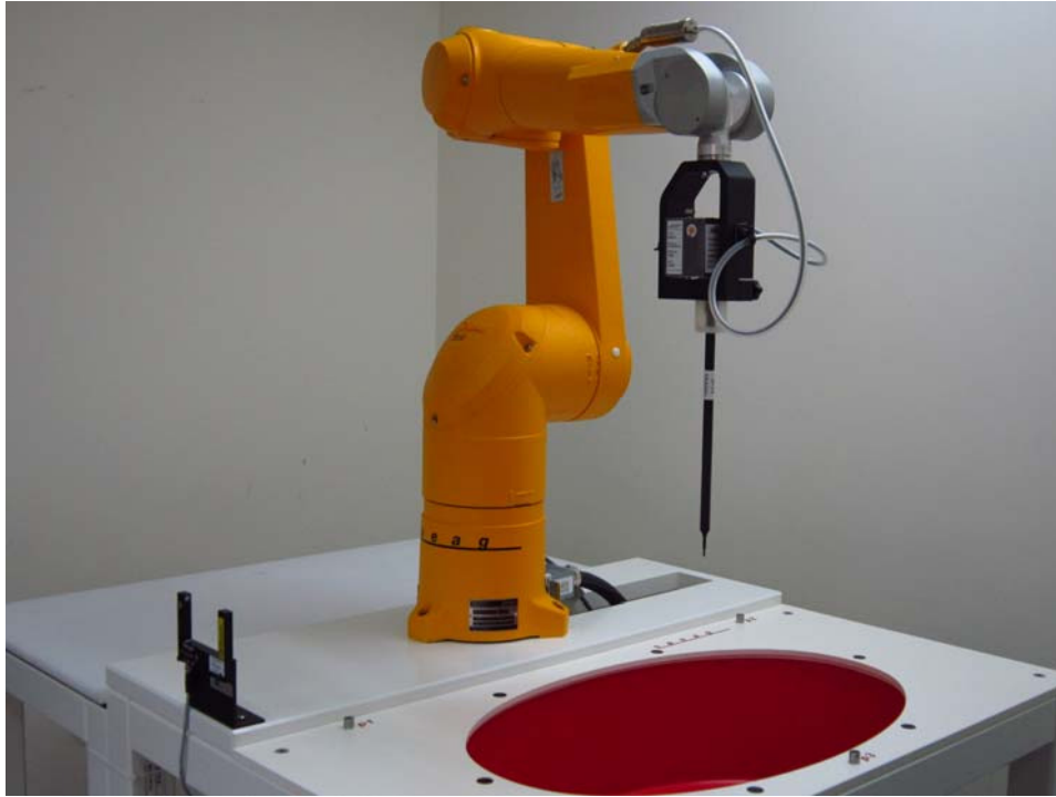
Fig.1 Photograph of the SAR measurement system
