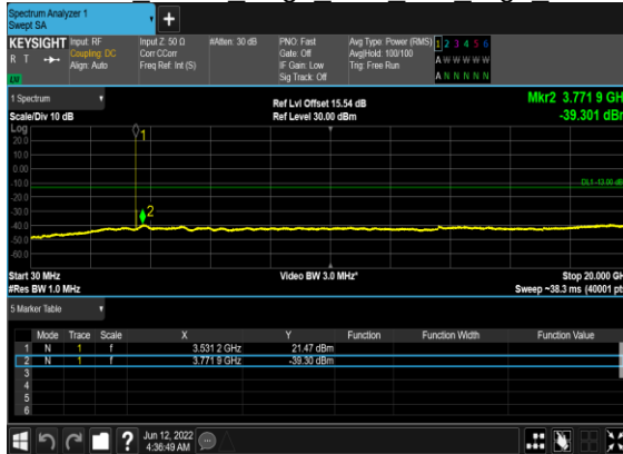
N78(20M)_DFT-s- OFDM BPSK Edge 1RB Left High CH
