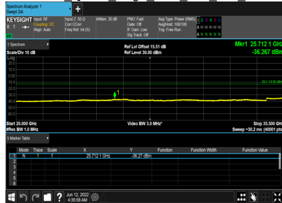
N78(20M)_DFT-s- OFDM QPSK Edge 1RB Left Mid CH
