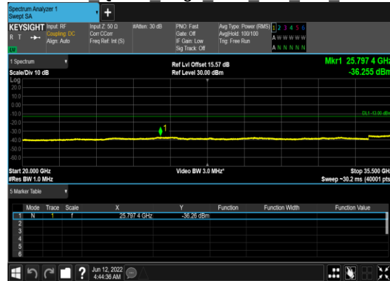
N78(60M)_DFT-s- OFDM QPSK Edge 1RB Left Mid CH
