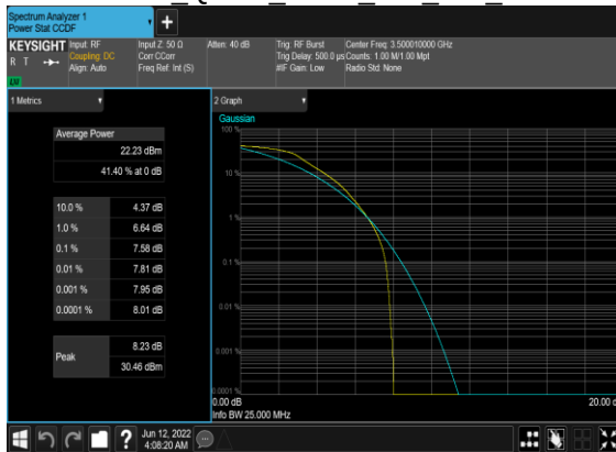
N78(20M)_DFT-s- OFDM QPSK Outer Full Mid CH
