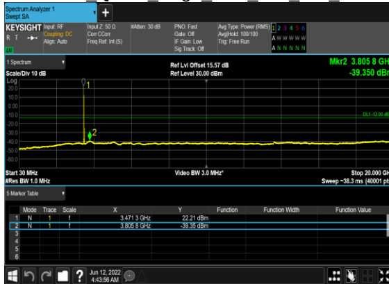
N78(60M)_DFT-s- OFDM QPSK Edge 1RB Left Mid CH
