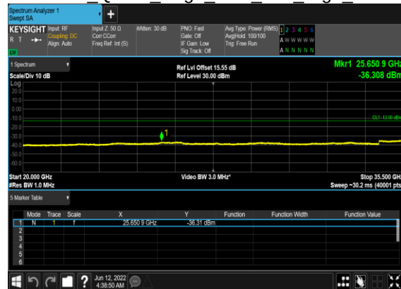
N78(20M)_DFT-s- OFDM QPSK Edge 1RB Left High CH
