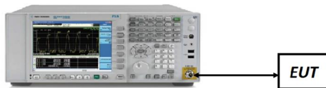
Figure 7-1. Test Instrument & Measurement Setup
