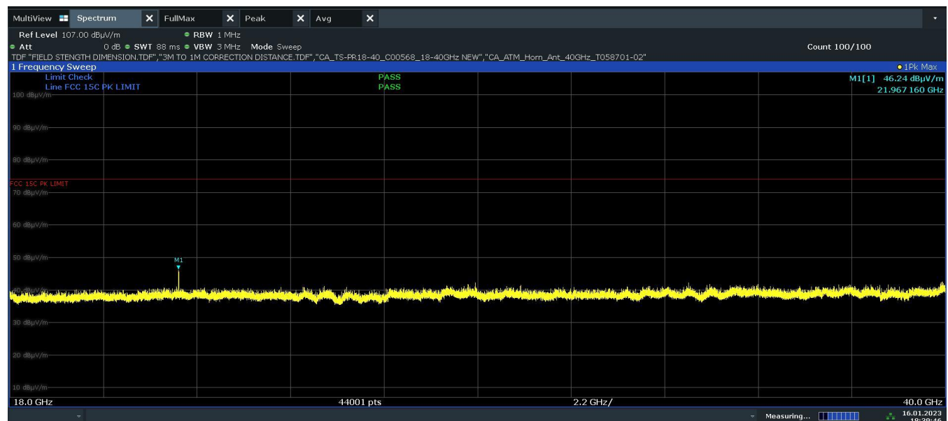
Plot 7-33. Radiated Spurious Emissions above 18GHz (BT GFSK - 2441MHz, Pol. V)
