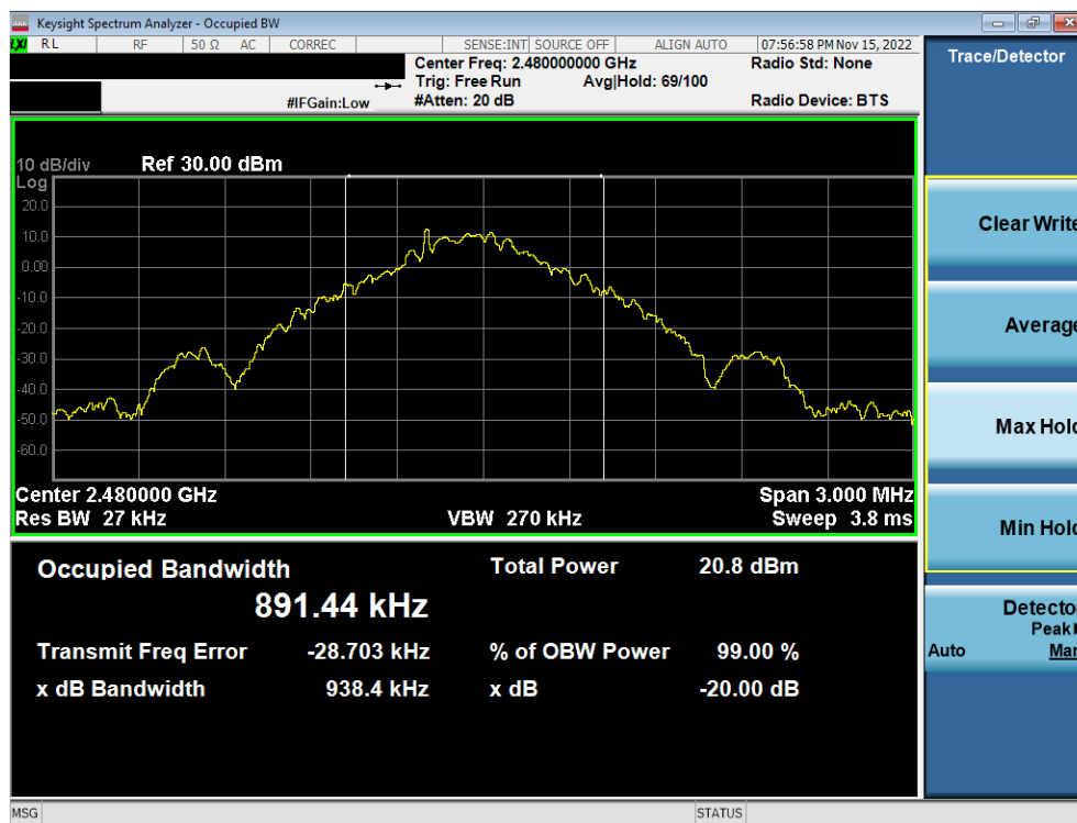
Plot 7-3. 20dB BW and 99% OBW Plot (Bluetooth, GFSK – 2480MHz)
