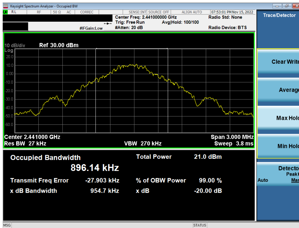
Plot 7-2. 20dB BW and 99% OBW Plot (Bluetooth, GFSK – 2441MHz)
