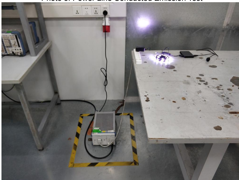
FCC ID: 2AQA6-H6104 Photo of Power Line Conducted Emission Test
