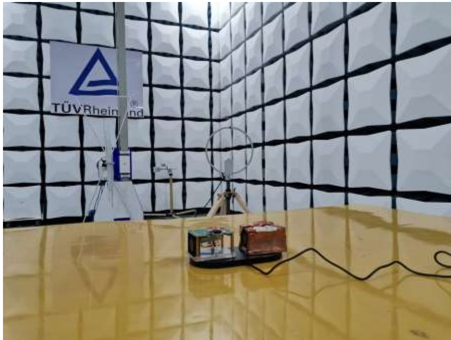
Photograph 1: Set-up photo for Radiated Emission, 9KHz - 30MHz
