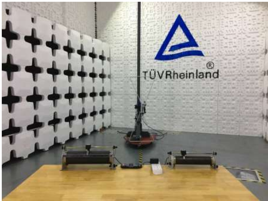
Photograph 2: Set-up photo for Radiated Emission, 30MHz - 1GHz
