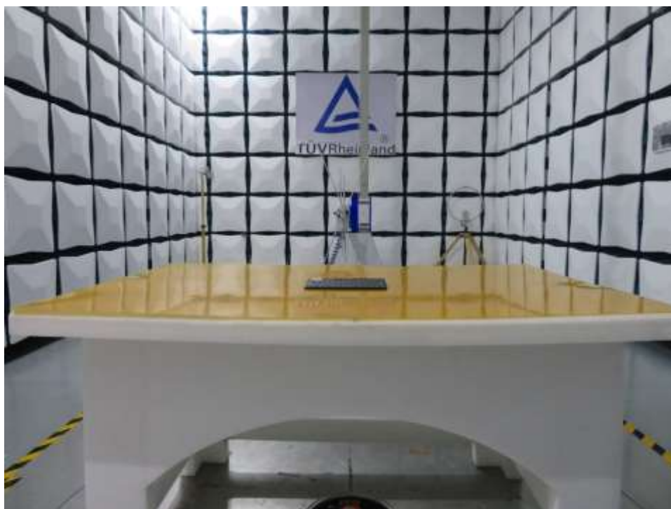
Photograph 1: Set-up photo for Radiated Spurious Emission, Below 1GHz
