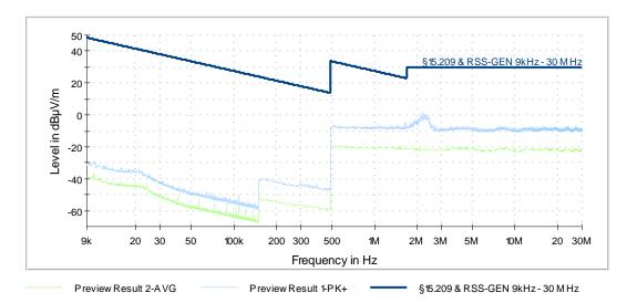
Remark: In the shown plot a distance correction factor was added to the measurement results to account for the different measuring distances according to standard (9 kHz to 490 kHz @ 300 m; 490 kHz to 30 MHz @ 30 m).
