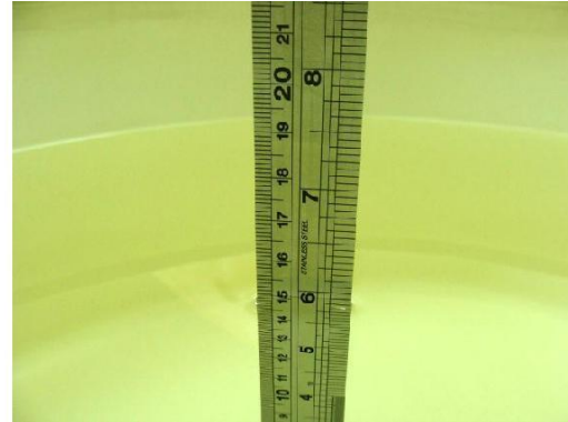
Fig 7.2 Photo of Liquid Height for Body SAR
