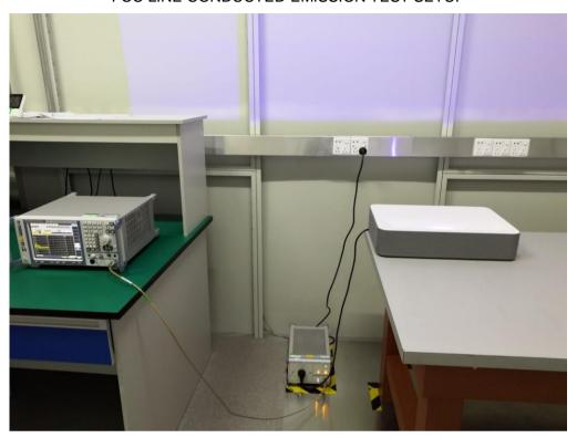
FCC RADIATED EMISSION TEST SETUP BELOW 1GHZ
