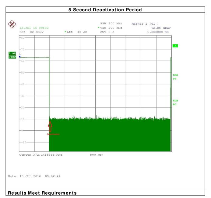
Test Data: Transmitter Deactivation Plot
