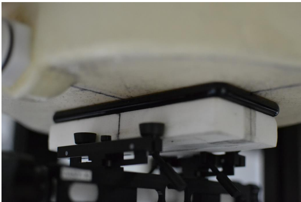
SAR Test Setup Photo 10 – Front Side at 0mm
