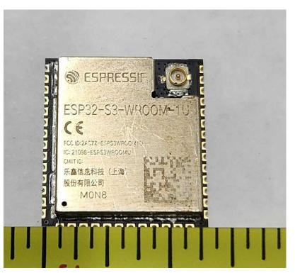
Espressif ESP32 Module with the label
