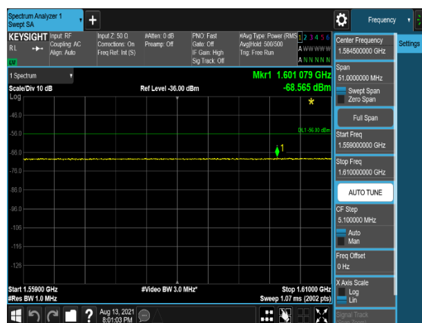
Plot 7-462. Conducted Spurious Emission Plot 1559 MHz to 1610 MHz (LTE_B13_10M+High_NB-Iot(GB)+Low_NB-Iot(IB)_2C_QPSK - Port 3)
